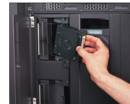
Mailslot design means you can add and remove cartridges easily without disrupting the system.
